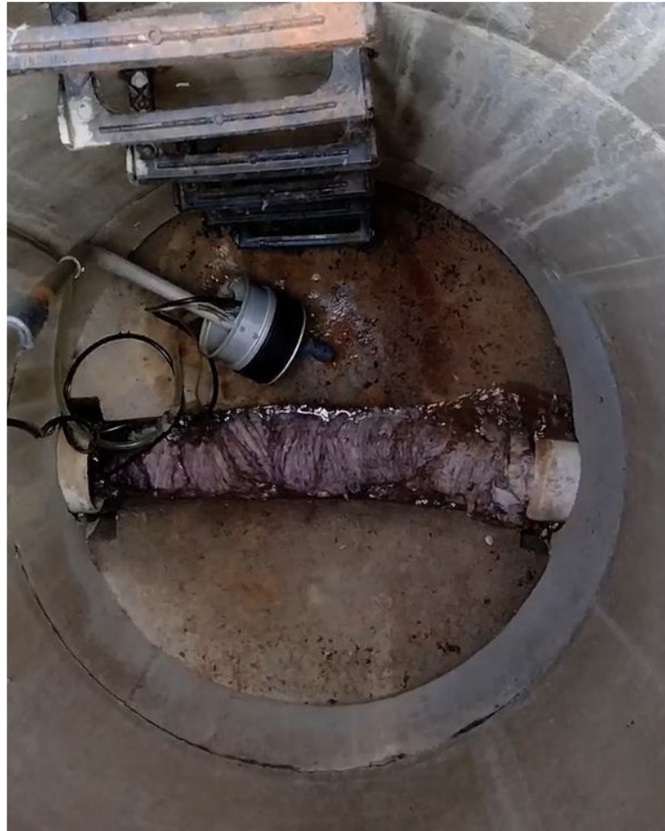
Weir removed from a sewage pipe following 24-hour composite sampling, showing a large number of rags flowing with industrial wastewater discharge.
