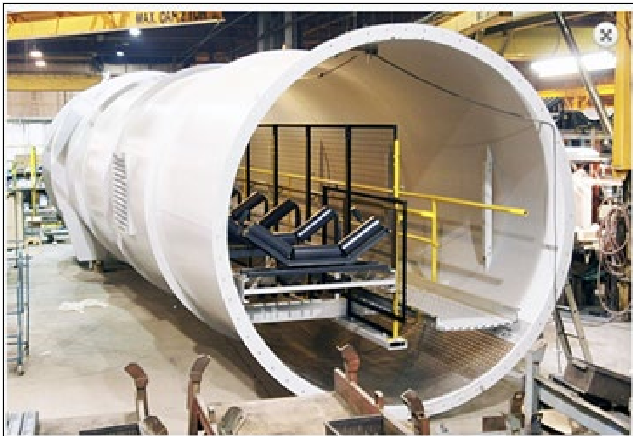
Figure 15: Conveyor Transport System with Tubular Gallery
