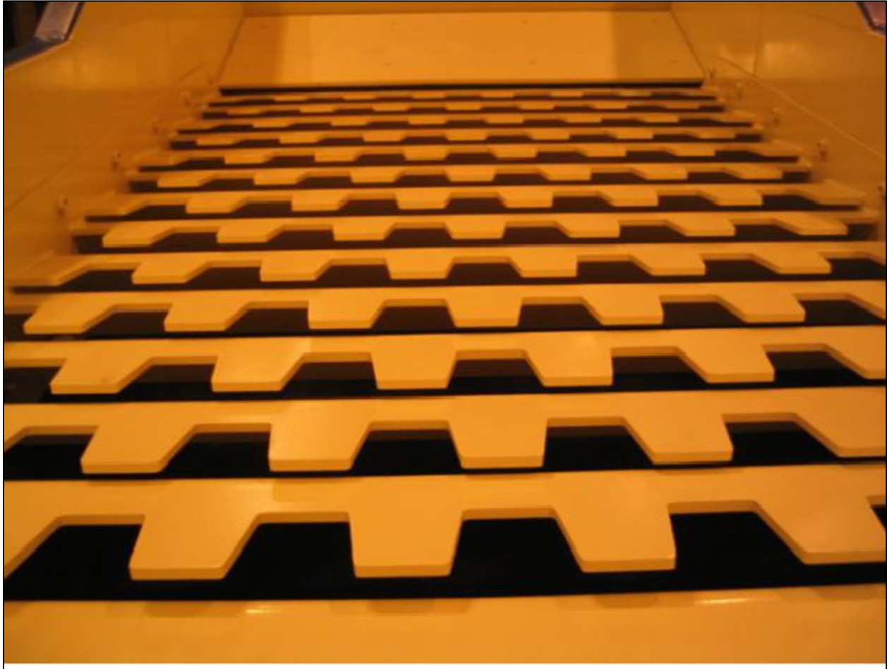
Figure 28: General Kinematics Grizzly Deck Design
