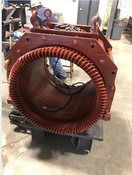
Pictured: Secondary Motor Rebuild
