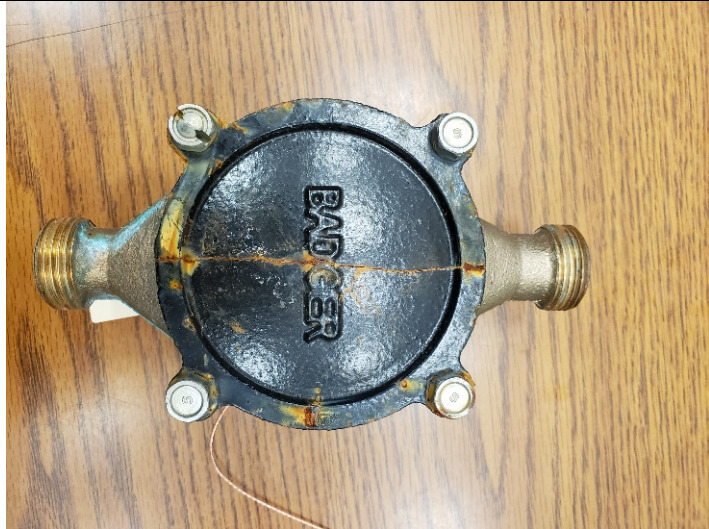
Photo of damaged meter from 5212 Lincoln Way
