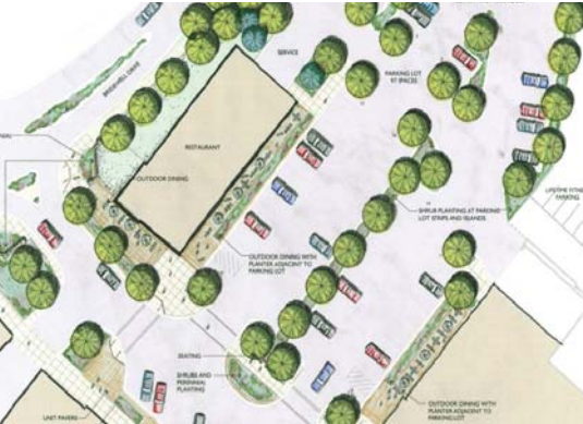
Parking rooms and landscaped screening, below left: Parking lots will be divided into 'rooms' or smaller blocks of parking spaces divided by landscaping. Landscaping should be designed to filter stormwater run-off, provide shade and screen the view of cars.
