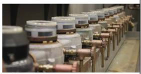
Water meters lined up on a test bench
