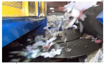
Figure 5: Disc Spreader
