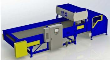
Figure 4: 3-D Typical Optical Sorter
