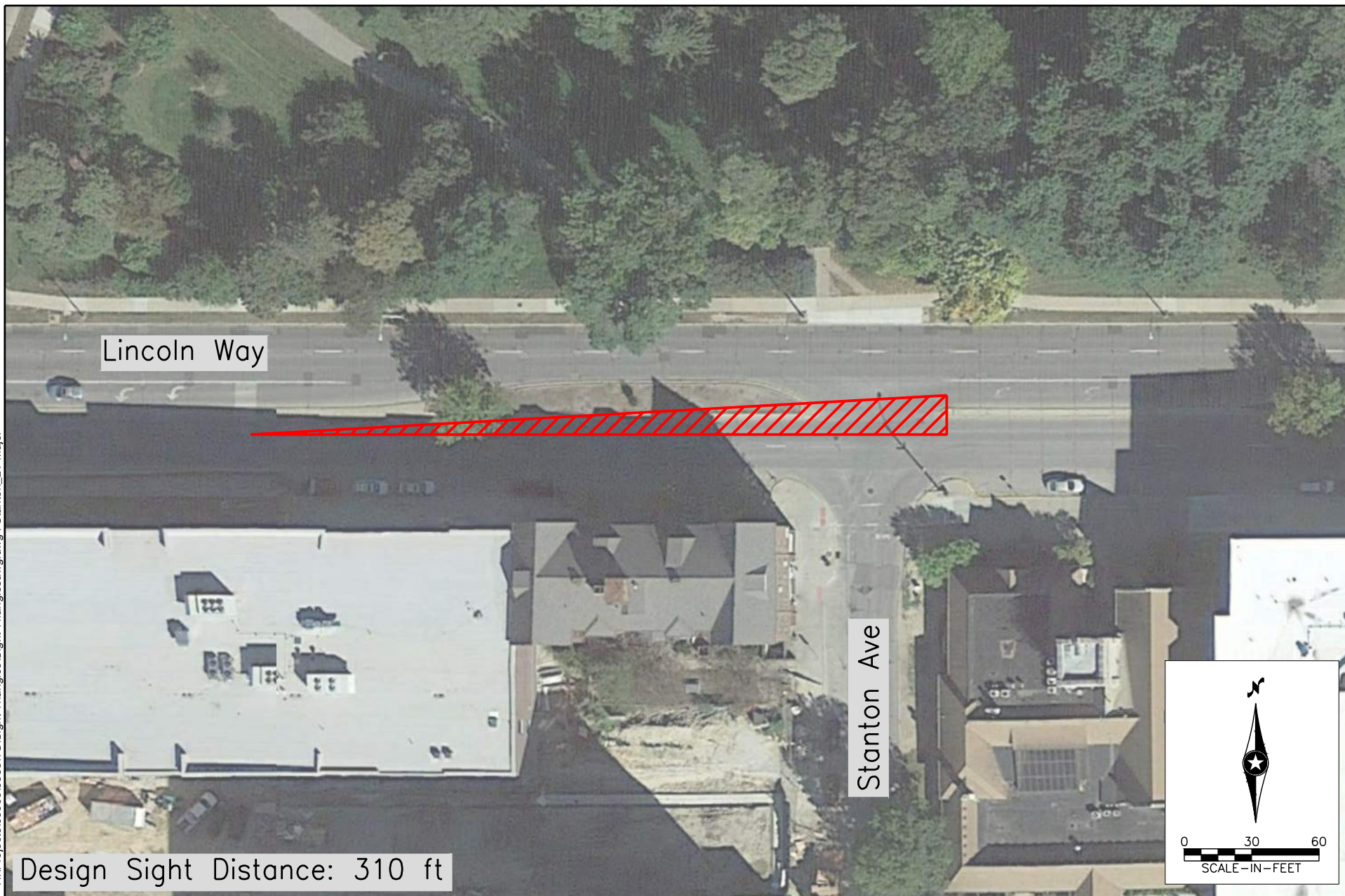
Lincoln Way & Stanton Ave Sight Triangles: Left-Turn from Major Approach Lincoln Way Safety and Operations Study Ames, Iowa
