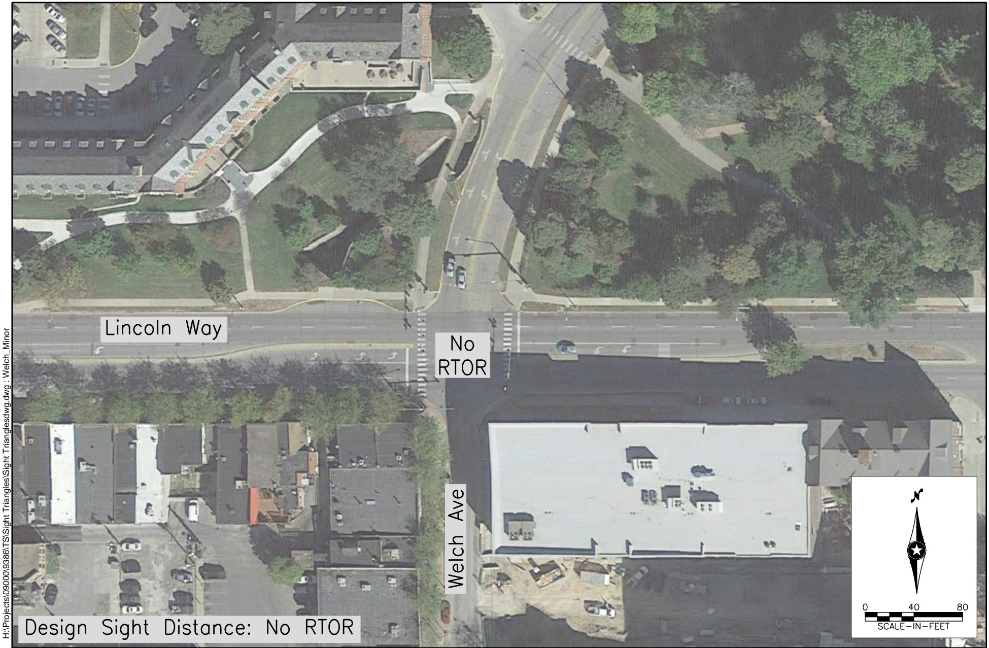
Lincoln Way & Welch Ave Sight Triangles: Right-Turn from Minor Approach Lincoln Way Safety and Operations Study Ames, Iowa
