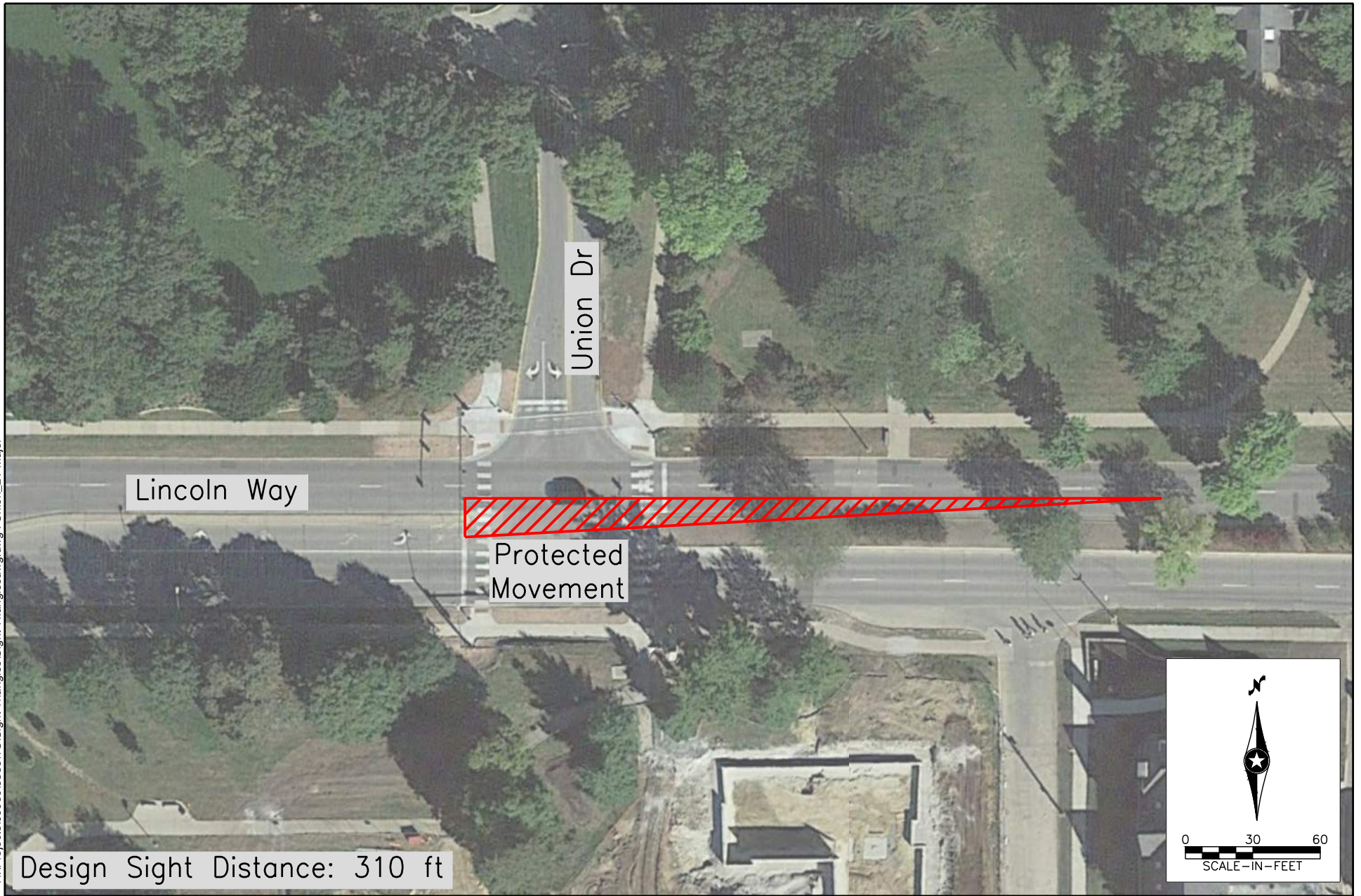
Lincoln Way & Union Dr Sight Triangles: Left-Turn from Major Approach Lincoln Way Safety and Operations Study Ames, Iowa
