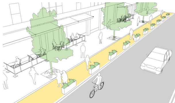
Example of closing parking spaces with planters for widened sidewalks, such as on east side of the 100 block of Welch Avenue
