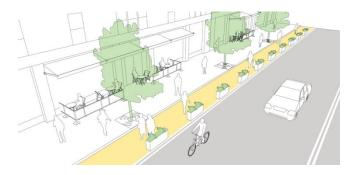
**Bike Corral** – A bike rack for 15-30 bicycles, placed on the street in a standard parking space. These structures could be placed seasonally or permanently. Placing a large bike corral on the street instead of several smaller racks can reduce streetscape clutter, but may be less convenient for bicyclists.
