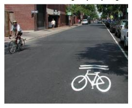
**Bike Lane** – A lane restricted to bicycles only, 4-5 feet in width and is designated for one-way travel. Roadways may have a bike lane in one direction, bike lanes in both directions, or a bike lane in one direction and a sharrow in the opposite direction.
