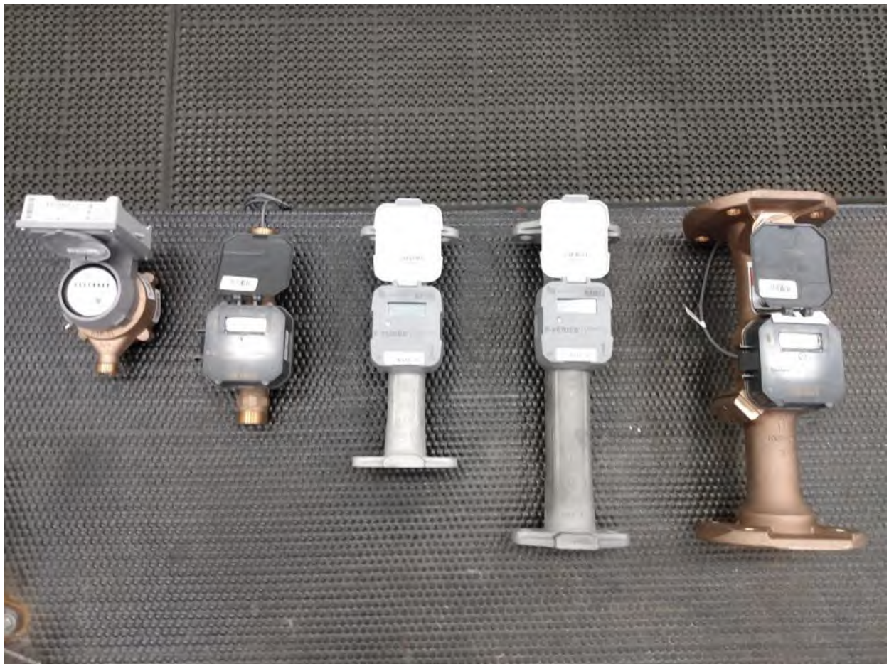
This photo shows the most common meter sizes from a 5/8"x3/4" mechanical residential meter up to a 3" commercial ultrasonic meter. They range in flow rates from .25 gpm up to 550 gpm.
