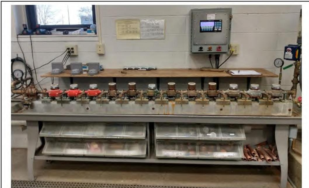
This photo shows a meter test bench in the Water Meter Laboratory full of 12 meters in the process of being tested.
