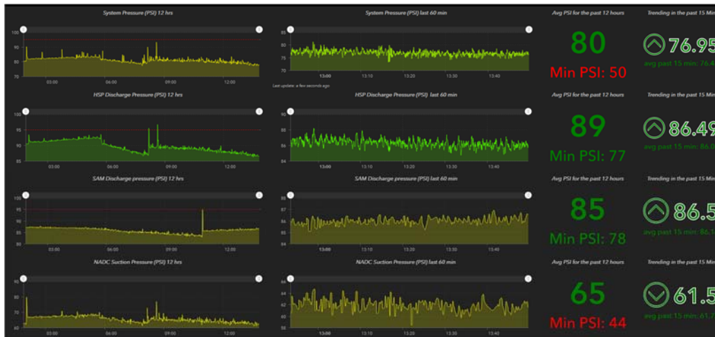
A mock-up of a pressure monitoring “dashboard” that will trend pressures in the distribution system and generate alarms for any unusual conditions.
