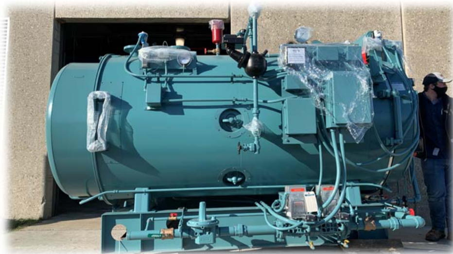
New dual-fuel boiler being delivered to WPC
