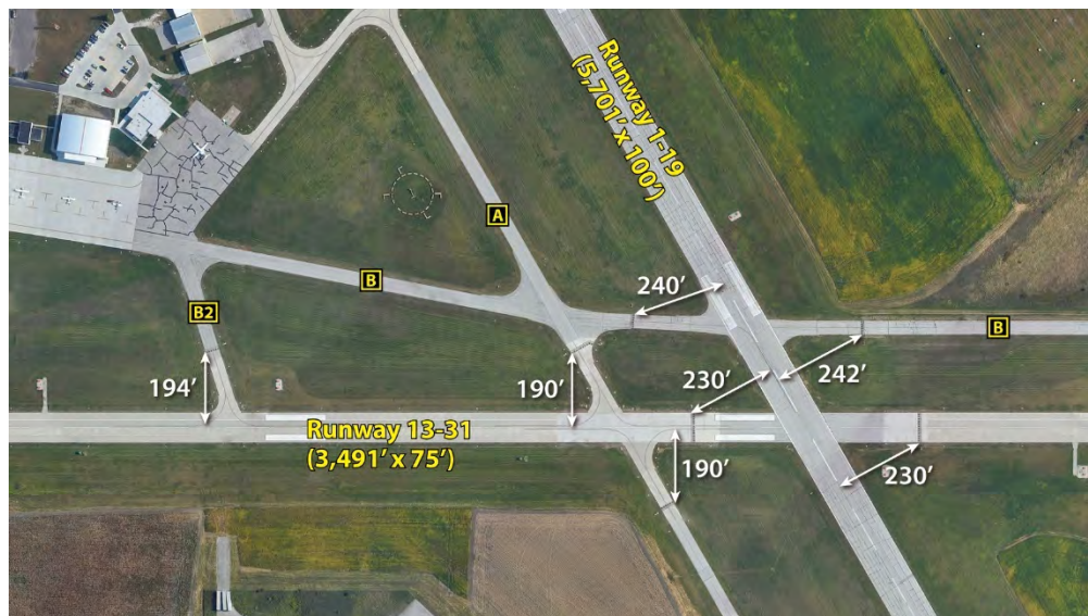
Figure 3A Holding Position Markings
