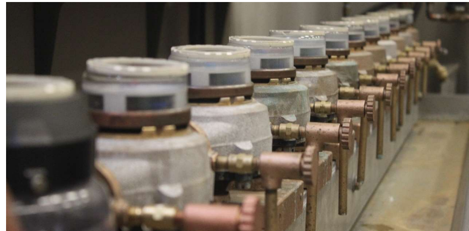
Water meters lined up on a test bench
