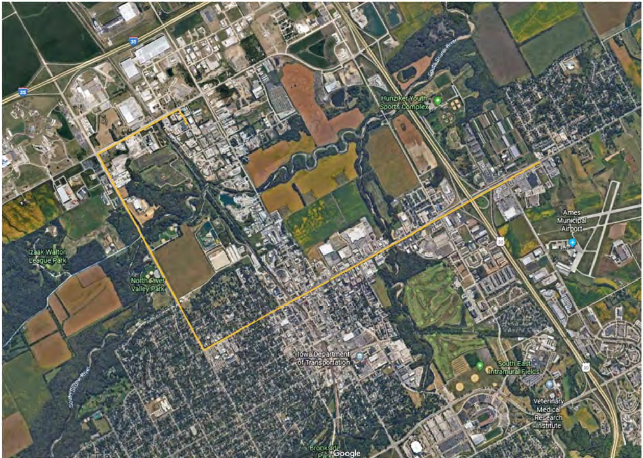
Figure 1 - First Phase Fiber Routing (shown in Yellow)
