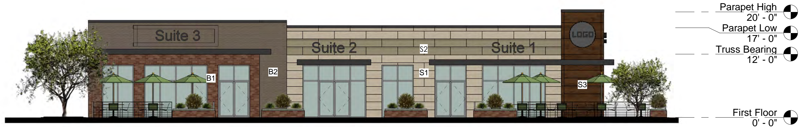
① East Elevation 3/32" = 1'-0"
