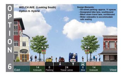
The additional feedback provided can be incorporated into this hybrid Option 6, such as new decorative light poles, trees, in-ground stormwater plantings, and bike racks. This Option 6 would be consistent with the Welch Avenue reconstruction project recently completed by ISU (bike lane southbound, sharrows northbound).
