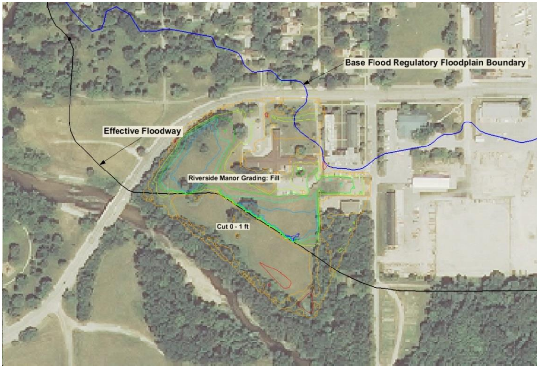
Figure 2: Riverside Manor Grading plan compared to effective floodway and base flood floodplain boundary
