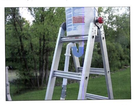
As I let the water in the 5-gallon bucket drain out, most of the water in the trap ended up getting siphoned out. I added some food coloring to the water and held my flashlight up against the back of the trap to show this.
