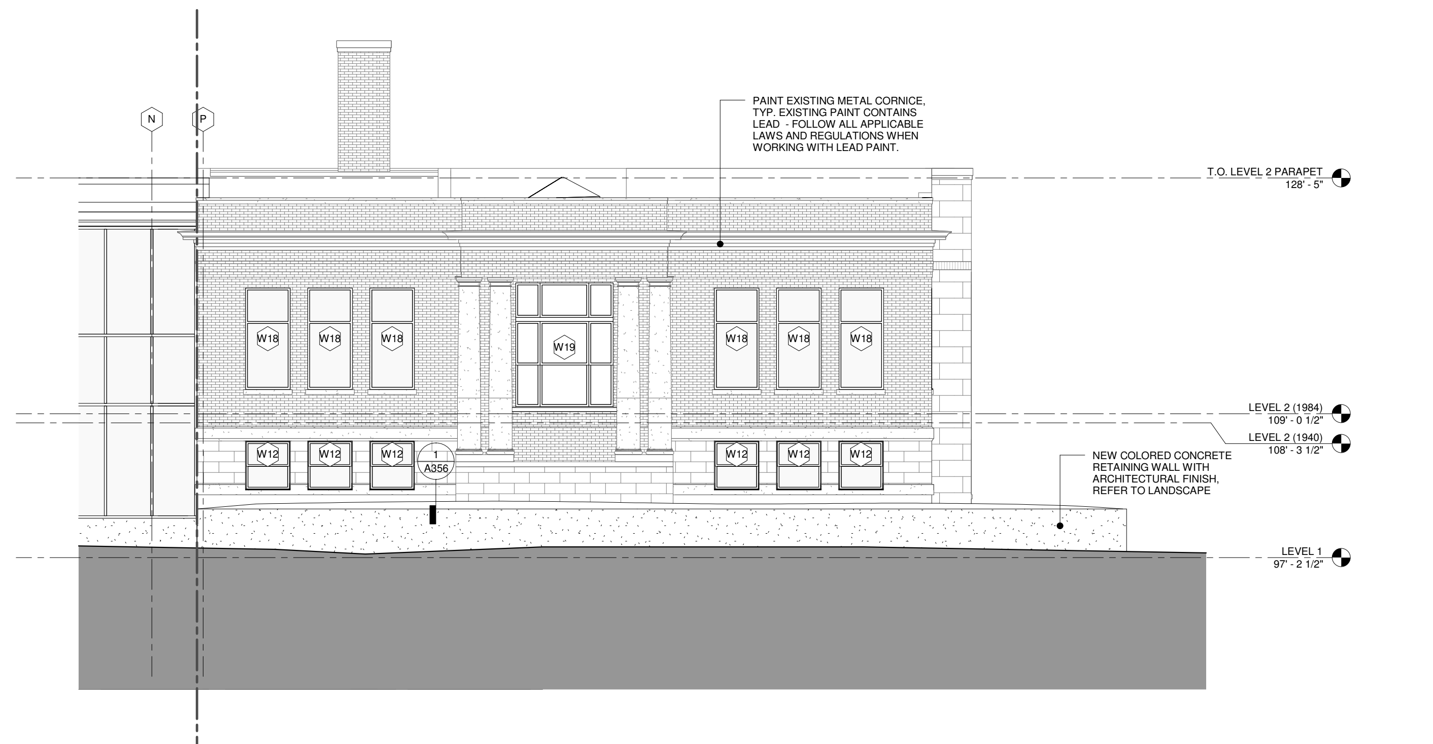
2 BUILDING EAST ELEVATION - NORTH A201 1/8" = 1'-0"
