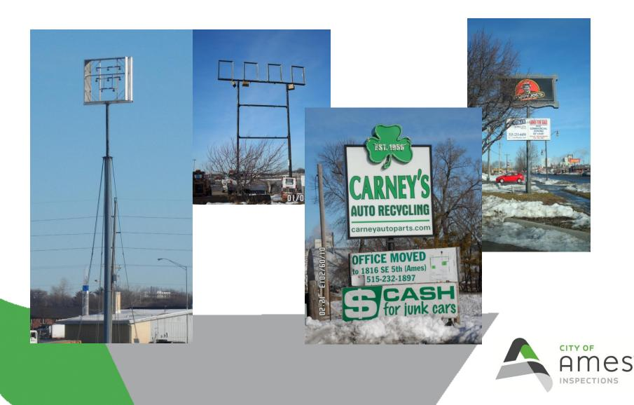
Change #2 – If sign is removed, the sign structure must have a new sign or a solid color blank panel. Implicitly allowed: removing the frame that holds the sig
