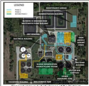
Conceptual layout of all phases of the Nutrient Reduction Modifications Project.
