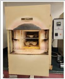
A photo of the muffle furnace.
